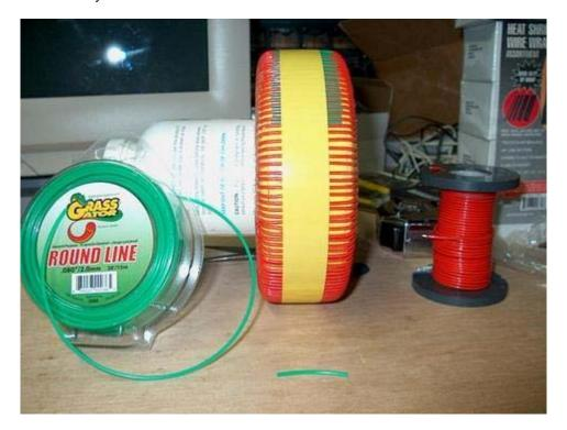
As you can see here, Bob uses short lengths of plastic strimmer cable as spacers for the outside of the toroid, though the picture above has been taken to show what a partially prepared secondary winding looks like when its windings are being moved into very accurate positions.
