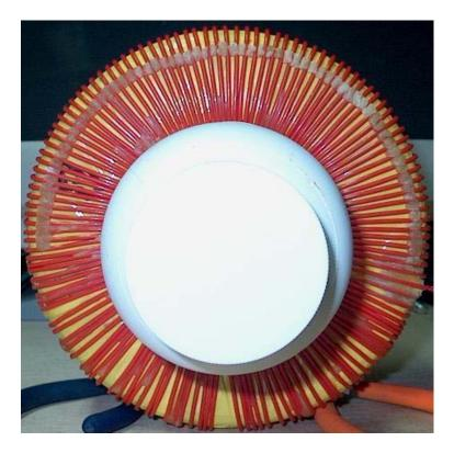
When the windings are completed, correctly spaced and encased in beeswax, each layer is finished off with a layer of tape.
